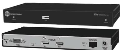
The compact Zio S2000 encoder accepts signals up to 4K resolution over a locking HDMI connector with loop through capability. The S2000 encodes video, audio, and control signals using industry standard compression. Power over Ethernet (PoE) is provided to simplify installation.
