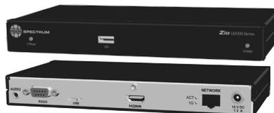
The compact Zio D2000 is a flexible decoder designed to work with the S2000 encoder and H.264/H.265 compliant devices. The D2000 decodes and displays streams at up to 4K resolution. Power over Ethernet (PoE) is provided to simplify installation.
