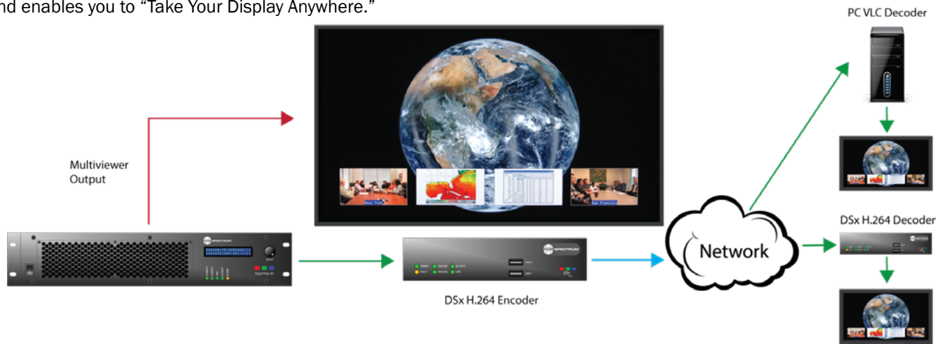
DSx Codec used as part of a remote monitoring system
