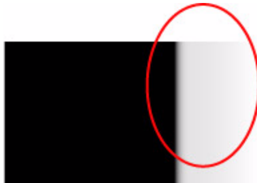
Figure 3-4. Streaking resulting from incorrect distance compensation
