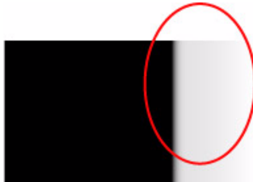
Figure 4-5. Alignment image with incorrect distance compensation
